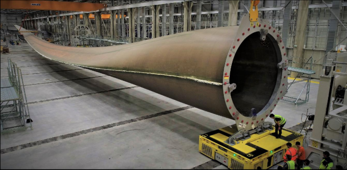
Modern plastic blade of a wind turbine: energy intensive to make, transport, and install. Difficult to recycle
